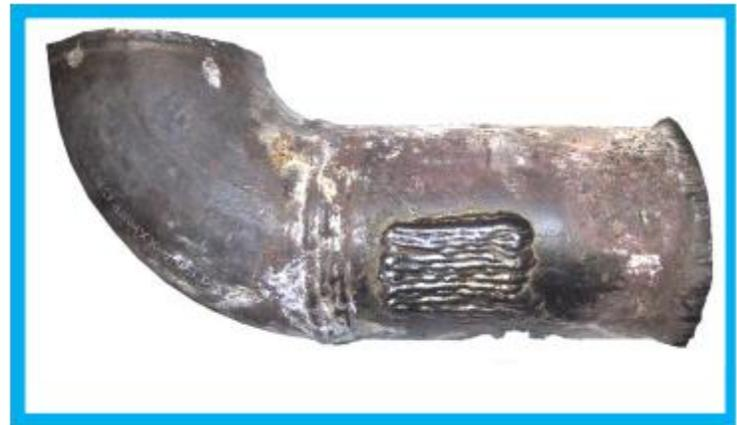
**Case History 1:** case history involving the installation of a total of six CRV<sup>®</sup>s, one upstream of each of six 2" extra heavy pipe elbows for wet steam service in a paper mill, prove successful operation for more than two years after installation. Previously, elbow replacement was required every 3 months.
