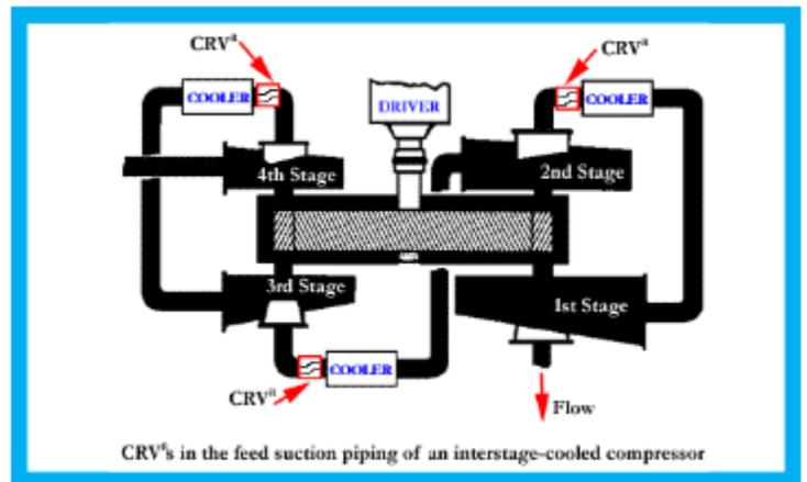
CRV<sup>®</sup>s in the feed suction piping of an interstage-cooled compressor
