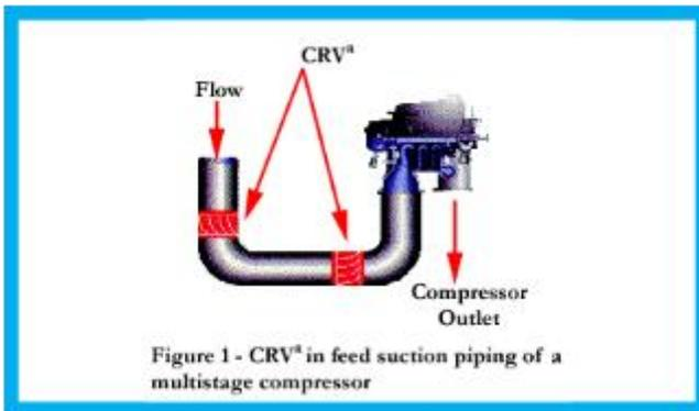
Figure 1 - CRV<sup>®</sup> in feed suction piping of a multistage compressor
